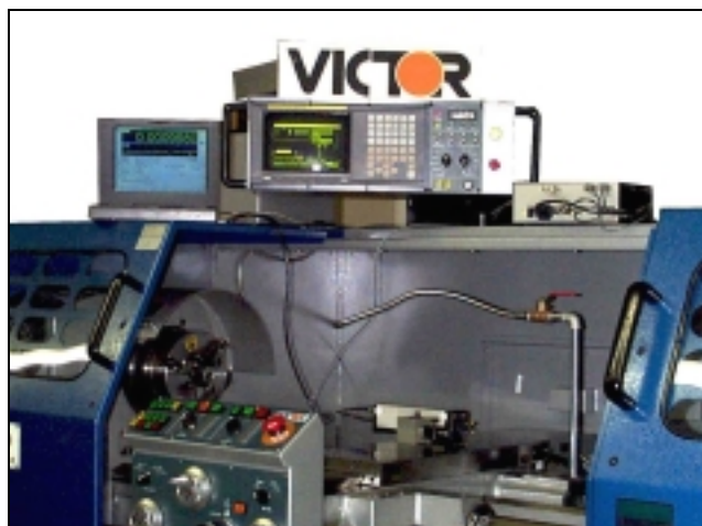
Victor 1860DCL X-Axis Laser Calibration Setup
